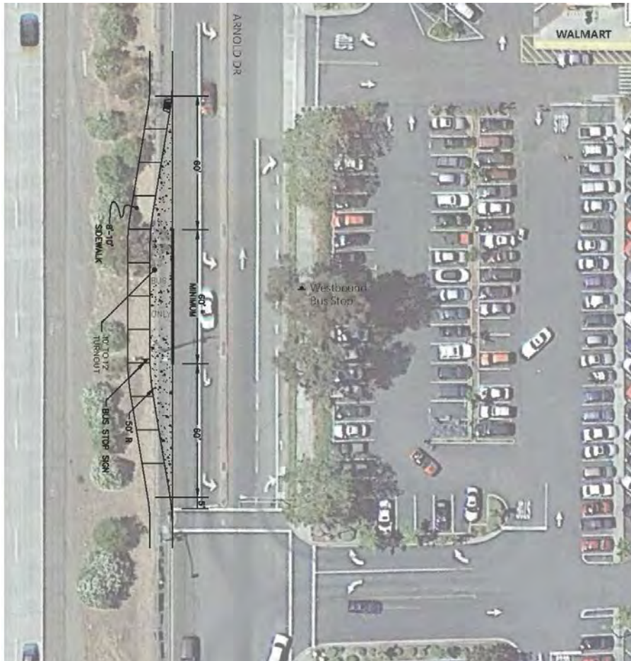
Figure 5-32 Arnold Drive Bus Turnout Design
