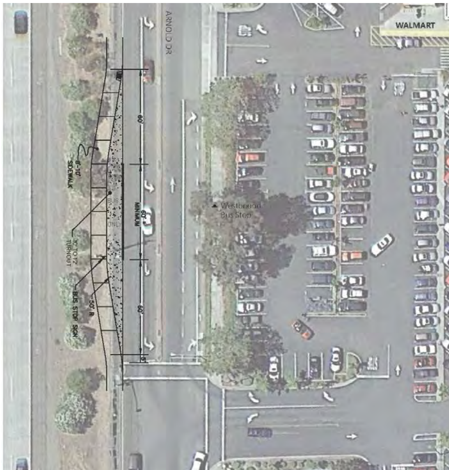
Figure 5-32 Arnold Drive Bus Turnout Design
