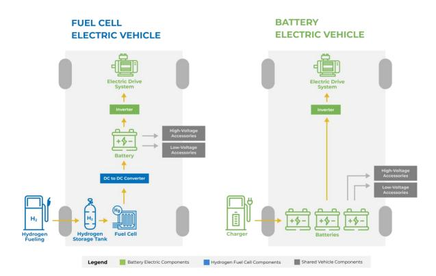
Figure 2- Battery and Fuel Cell Electric Bus Schematic
